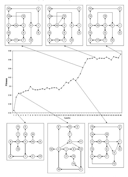
Fig. 3. The evolution of a robust rhythmic architecture with samples taken at different points. Central inset: plot of fitness vs. number of generations. A ring is formed early on; increases in fitness correspond to changes of the size of the ring and the distribution of Boolean functions.
