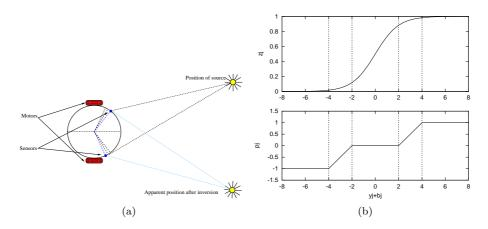
Figure 3: Experimental scheme: (a) agent body and effect of sensor swapping; (b) facilitation of local plasticity as a function of 'cell potential' (y). Top: neuron activity ('firing rate'). Bottom: strength and sign of local plastic facilitation.
