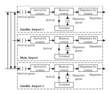
Fig. 3. Arrival-departure scheme of a three-airport system.
