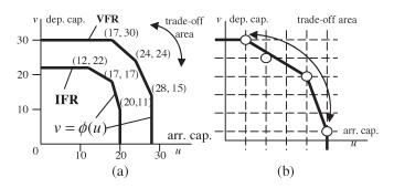
Fig. 4. Airport arrival-departure capacity curves (15 min).
