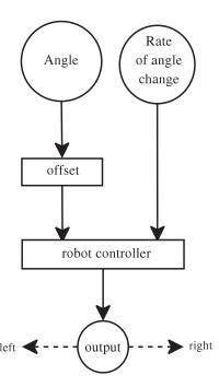
**Figure 6** The controller has an added mutable offset to compensate for the angle of the pole. This is added to the signal from the angle sensor before being fed into the rest of the controller.
