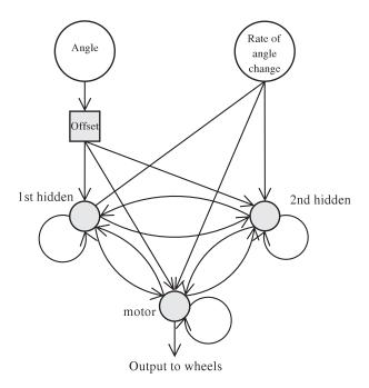
**Figure 7** The topology of the neural network remains static during the evolutionary run. Initially animats are evolved without a mutable offset, then with one mutable offset, and finally with two. This diagram shows a single offset.
