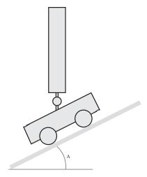
**Figure 5** The robot has to balance the pole whilst on an incline of 30°. The angle sensor no longer provides a signal of zero if the pole is balanced.
