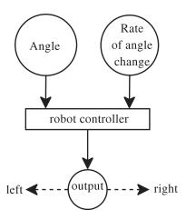
**Figure 4** Two inputs are fed directly into the controller. The controller decides whether the robot should move left or right and specifies the force in order to ensure the pole remains balanced. The pole has a mass of 5 kg and the cart of 1 kg. Gravity has a force of 2 ms<sup>-2</sup>.
