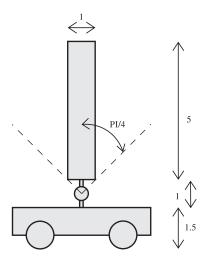
**Figure 3** The robot consists of a cart and a pole attached by a hinge joint. The hinge can swing freely and the pole is balanced in the vertical position. A robot succeeds if it can maintain the pole within  $\frac{\pi}{4}$  radians of the vertical. The permitted extent of the poles swing is shown by the dashed line.
