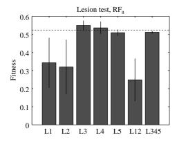
Fig. 9. Performance with lesioned  $RF_a$ , 'L1' denotes the performance of the robot when the first hidden neuron was lesioned; 'L345' when units 3, 4, and 5 were lesioned simultaneously. Fitness values are averaged over ten tests. This figure shows that the first and second hidden neurons play an important role for the performance of the robot. Horizontal dashed line represents the fitness value of the robot with intact receptive fields.
