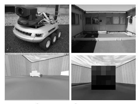
Fig. 2. Top left: The Koala mobile robot by K-Team with pan/tilt camera by Sony. Top right: The real environment. Bottom left: simulation of the robot and the environment. Bottom right: view from the simulated camera. The robot is capable of visually accessing the  $5 \times 5$  pixels in the center of the image.
