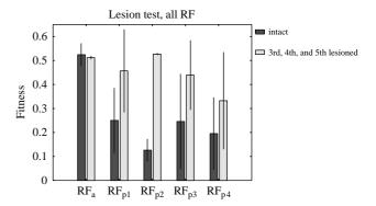
Fig. 10. Performance with lesioned receptive fields. Dark gray bar shows the performance with five intact receptive fields, whereas light gray bar with three lesioned neurons. The fitness values are averaged over 10 tests. The performances with all of  $RF_{p1-4}$  were improved by lesioning units 3,4, and 5.
