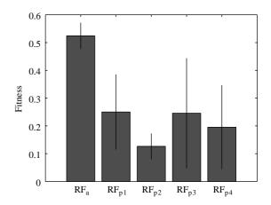
Fig. 7. Performances of the robot with receptive fields developed in active  $(RF_a)$  and passive  $(RF_{p1-4})$  conditions. The fitness values are averaged over ten tests. Vertical lines show the standard error.
