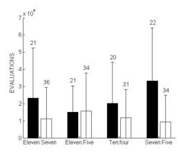
**Fig. 2.** Mean and standard deviations (error bars) of fitness evaluations required to evolve successful networks for each CPG pattern, Eleven-Seven, Eleven-Five, Ten-Four and Seven-Five. Black bar shows original mean data and white bar shows NSGasNet mean data. The numbers above each error bar represent the total number of successfully evolved networks within 50 runs.
